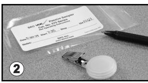
5. Write the stop time on the label on the pouch.
