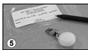
3. Remove the cap on the front of the sampler and set aside. **Do NOT remove the plastic plug on the back of the sampler. Removing this plug will VOID the sample.** Clip the sampler to the worker's clothing in the breathing zone. Ensure small holes are facing out. **Ensure holes are not covered in any way. Do not expose to rain/spray or splashing chemicals. Do not handle with dirty fingers/gloves.**
